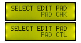
The DITI has a dedicated input for HiHAT control. It is input 7. When editing Trigger Input 7, you will see the name "padCTL" instead of the name 7A. This A input is designed for Continuous Controller HiHAT pedals. This input uses the tip for hihat control, so a mono 1/4" cable will function.
