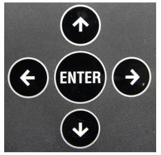
In Play Mode, the Up Down Arrows Changes the KIT TYPES, that is the name of the sound module that you are using.
